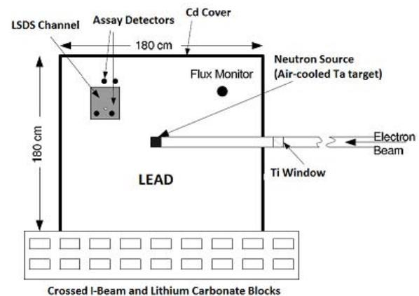
Figure 1: Diagram of RPI LSDS
