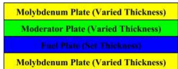
**Figure 3: Schematic of a unit cell.**
