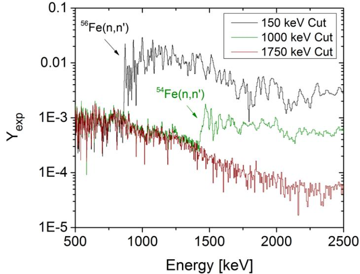
**Figure 2.** Capture yields in iron from 500-2500 keV, showing the effects of applying energy discriminators above the inelastic thresholds of  $^{54,56}\text{Fe}$ .
