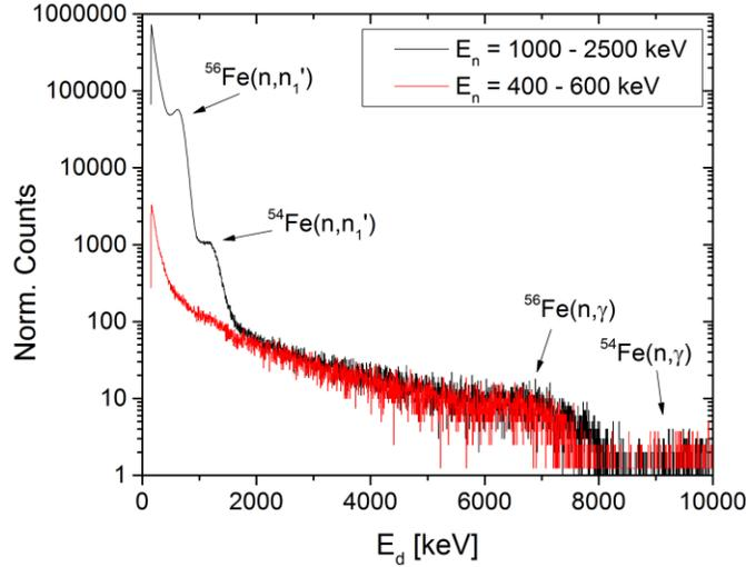
**Figure 1. Photon energy spectra above and below the inelastic thresholds of  $^{54,56}\text{Fe}$ .**
