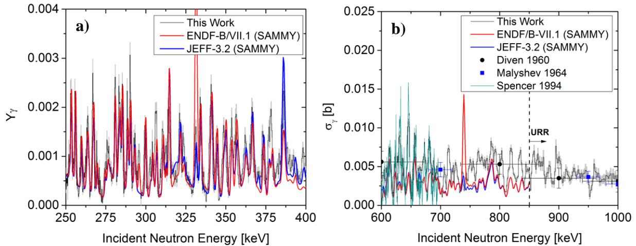
**Figure 3.** Comparison of capture yields in elemental iron from experimental data and existing evaluations in the energy ranges a) 250-400 keV; b) 600-1000 keV.
