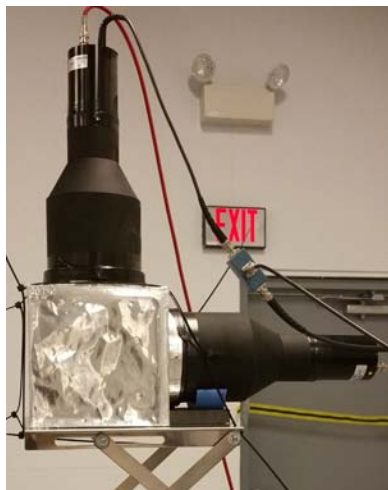
Fig. 1. Image of the in-beam neutron flux monitor placed in the neutron beam and situated far from the detector setup to avoid scattering into the capture detection setup.
