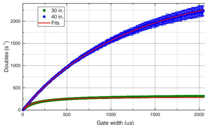
**Fig. 4.** Sample doubles fits from the LANL <sup>3</sup>He neutron multiplicity detector at different simulated water heights. Simulations were performed w/MCNP<sup>®</sup>6, and the fits were generated using Origin<sup>®</sup>.
