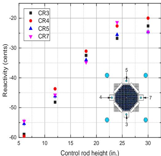
**Fig. 3.** Simulated reactivity worth curves for the RPI-RCF control rods. The simulation geometry is also included. The simulated curves will be compared to experimental control rod worth curves of the proposed configuration after the experiment is conducted.
