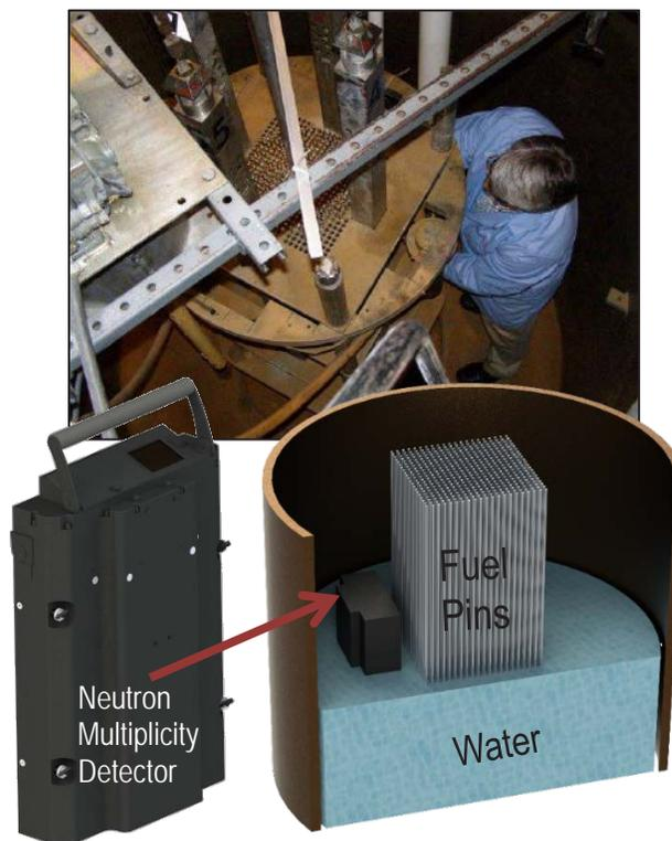
**Fig. 1.** Photograph of the RPI-RCF (above), and a Solidworks® simplified graphic rendering of the CaSPER measurement campaign at the RPI-RCF (below).
